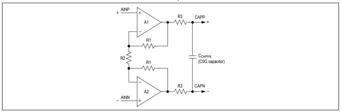
Figure 2. Simplified Equivalent Diagram of the PGA
