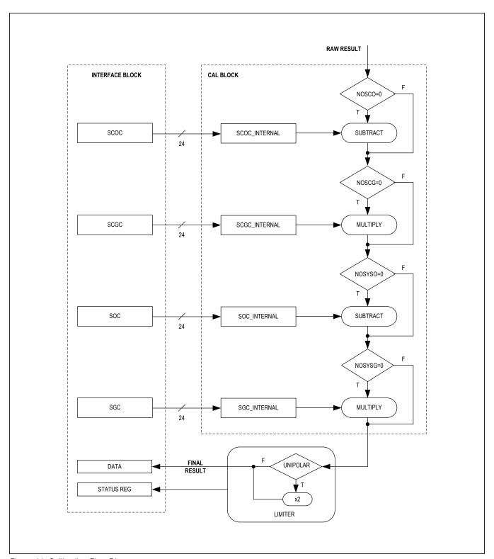
Figure 14. Calibration Flow Diagram
