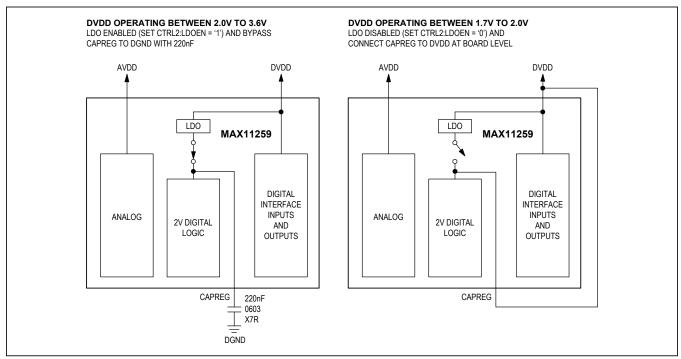
Figure 9. MAX11259 Digital Power Architecture
