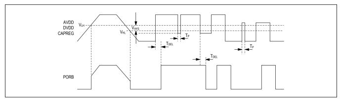
Figure 10. Undervoltage Lockout Characteristic Voltage Levels and Timing
