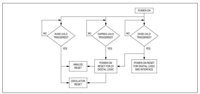
Figure 11. MAX11259 UVLO and POR Flow Diagram
