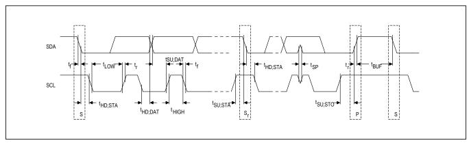
Figure 1. I<sup>2</sup>C Timing Diagram
