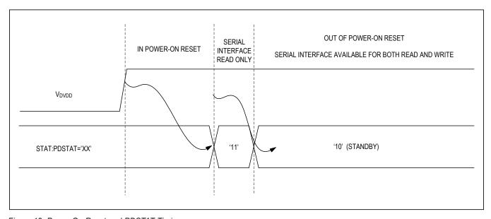
Figure 12. Power-On Reset and PDSTAT Timing
