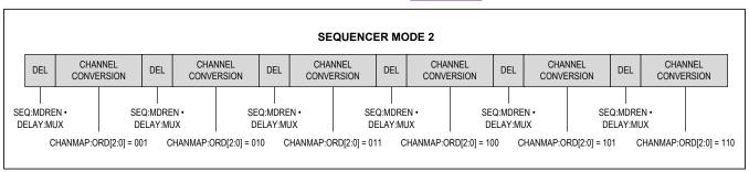
Figure 7. Sequencer Mode 2 Timing Diagram
