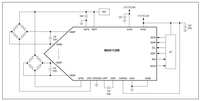
Figure 19. Application Diagram for 1.8V DVDD
