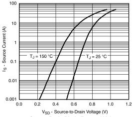
**Source Drain Diode Forward Voltage**
