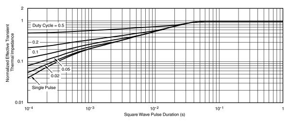
Normalized Thermal Transient Impedance, Junction-to-Case
