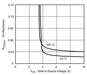
On-Resistance vs. Gate-to-Source Voltage
