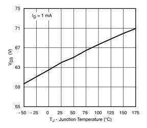
**Drain Source Breakdown vs. Junction Temperature**
