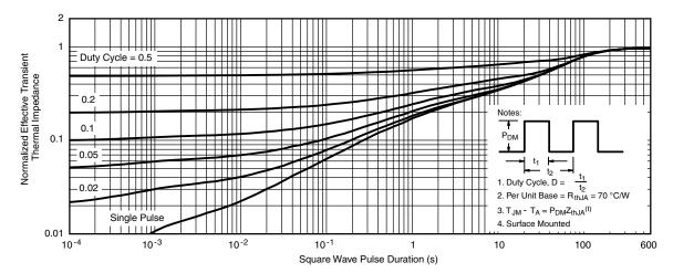
Normalized Thermal Transient Impedance, Junction-to-Ambient
