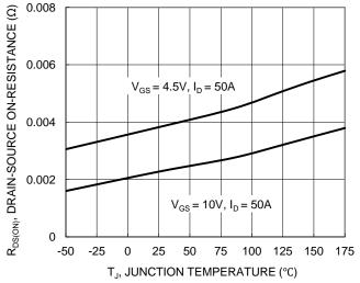
Figure 7. On-Resistance Variation with Temperature
