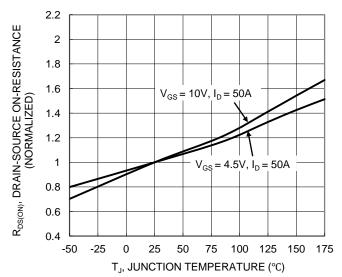
Figure 6. On-Resistance Variation with Temperature
