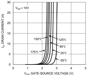
V<sub>GS</sub>, GATE-SOURCE VOLTAGE (V) Figure 2. Typical Transfer Characteristic
