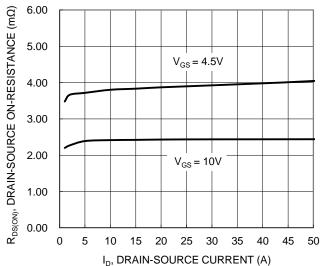
Figure 3. Typical On-Resistance vs. Drain Current and
