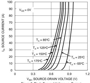
Figure 9. Diode Forward Voltage vs. Current
