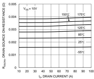
Figure 5. Typical On-Resistance vs. Drain Current and Temperature
