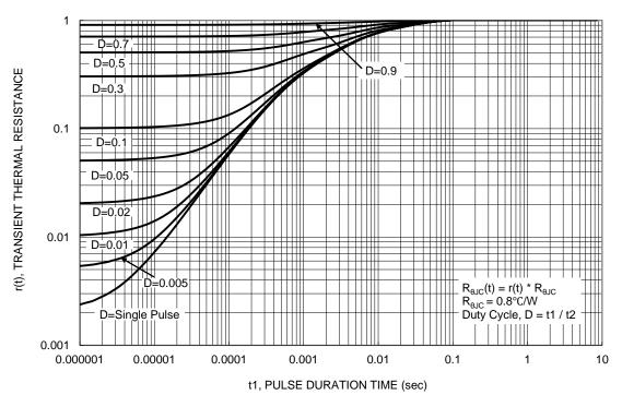
Figure 13. Transient Thermal Resistance
