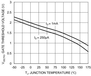
Figure 8. Gate Threshold Variation vs. Temperature
