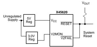
**Notice:** No external components required to monitor two voltages.
