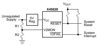
R1 and R2 selected so V2 = V2MON threshold when Unregulated supply reaches 6V.
