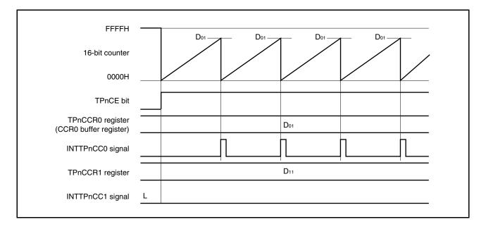
Figure 6-25. Timing of Operations When D<sub>01</sub> < D<sub>11</sub>
