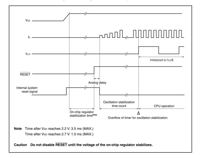
Figure 22-3. Timing of Power-on Reset Operation
