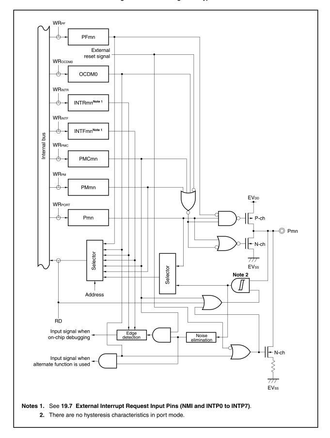
Figure 4-36. Block Diagram of Type AA-1
