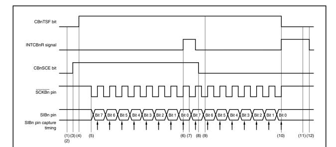
Figure 16-26. Continuous Transfer Mode Operation Timing (Slave Mode, Reception Mode)
