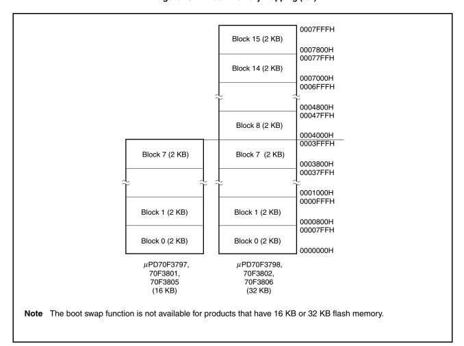
Figure 28-1. Flash Memory Mapping (1/2)
