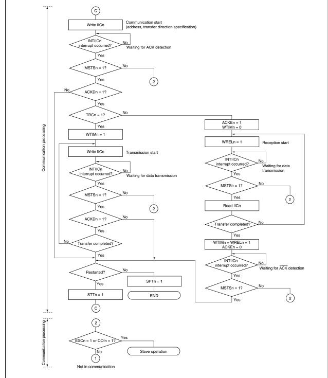
Figure 17-19. Master Operation in Multimaster System (3/3)
