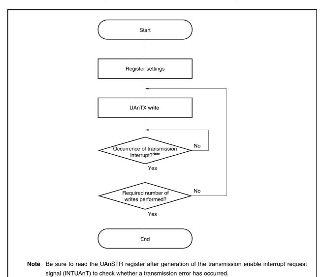
Figure 15-7. Continuous Transmission Processing
