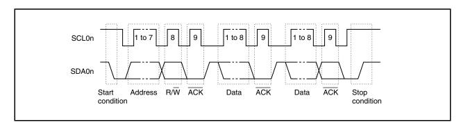
Figure 17-7. I2C Bus Serial Data Transfer Timing
