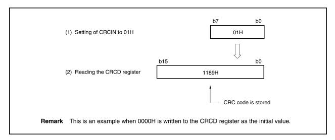
The code when 01H is sent LSB first is (1000 0000). Therefore, the CRC code calculated by using the generation polynomial  $X^{16} + X^{12} + X^5 + 1$  is the remainder when sixteen digits of zero are appended to (1000 0000) to make the code become (1000 0000 0000 0000 0000 0000) and the code is divided by (1 0001 0000 0010 0001) by using a modulo-2 operation formula.
