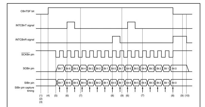
Figure 16-28. Continuous Transfer Mode Operation Timing (Slave Mode, Transmission/Reception Mode)
