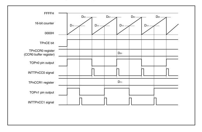
Figure 6-14. Timing of Operations When D<sub>01</sub> ≥ D<sub>11</sub>
