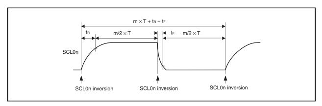
The clock to be selected can be set by the combination of the SMCn, CLn1, and CLn0 bits of the IICCLn register, the CLXn bit of the IICXn register, and the OCKSTHm, OCKSm1, and OCKSm0 bits of the OCKSm register (m = 0, 1).
