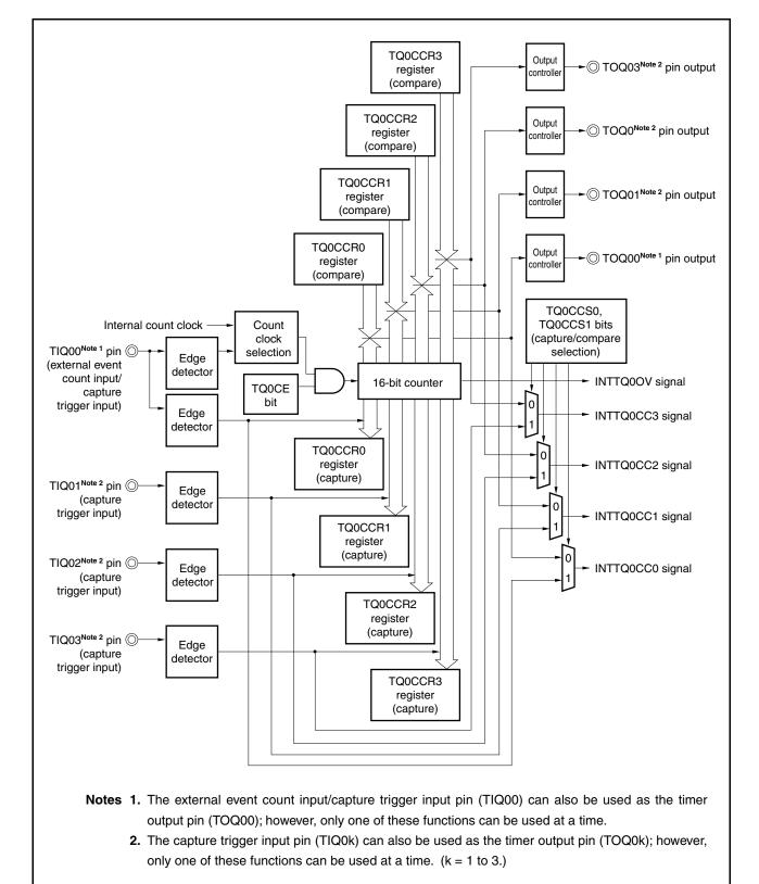
Figure 7-52. Configuration of TMQ0 in Free-Running Timer Mode
