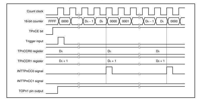
Figure 6-32. Outputting 100% PWM Waveform
