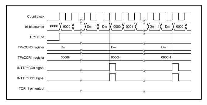
To output a 100% waveform, set the value of TPnCCR0 register + 1 to the TPnCCR1 register. If the value of the TPnCCR0 register is FFFFH, a 100% waveform cannot be output.
