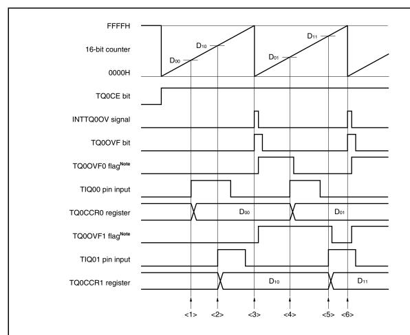
Note The TQ0OVF0 and TQ0OVF1 flags are set on the internal RAM by software.
