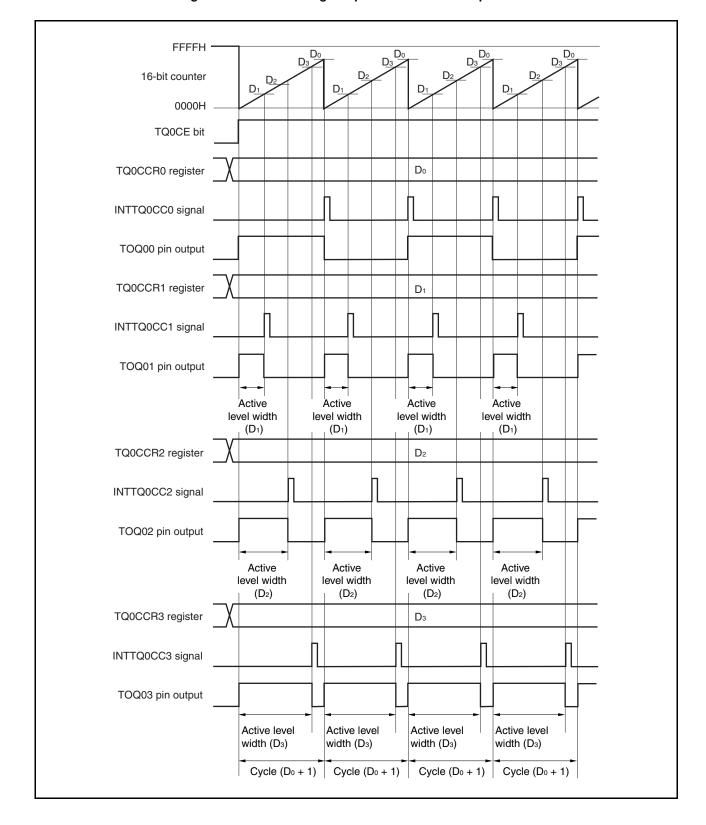
Figure 7-45. Basic Timing of Operations in PWM Output Mode
