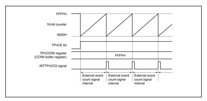
Figure 6-21. Operation When TPnCCR0 Register Is Set to FFFFH
