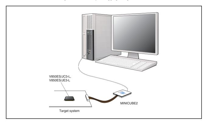
Figure 29-1. On-Chip Debugging Using MINICUBE2
