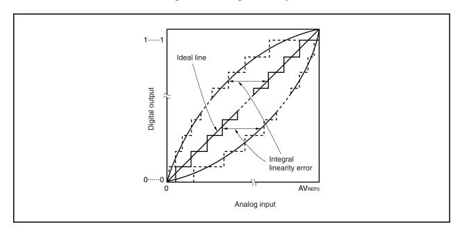
Figure 13-21. Integral Linearity Error
