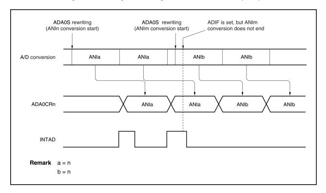
Figure 13-13. Timing of Generating A/D Conversion End Interrupt Request
