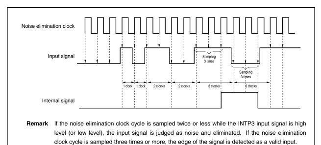
Figure 19-15. Example of Digital Noise Elimination Timing
