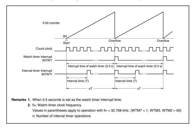
Figure 9-2. Timing of Watch Timer and Interval Timer Operations
