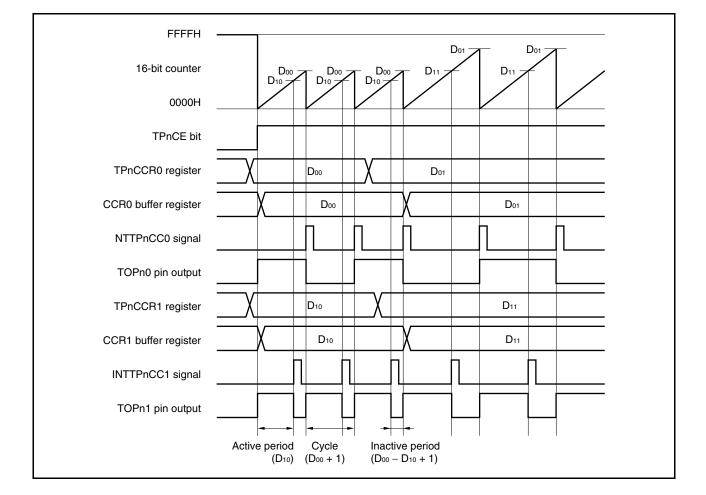
Figure 6-45. Basic Timing of Operations in PWM Output Mode
