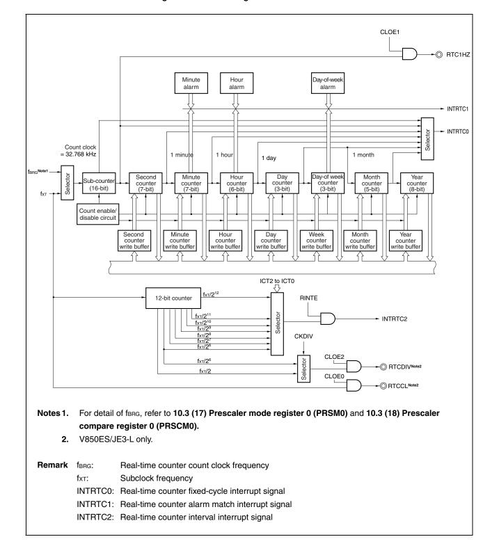
Figure 10-1. Block Diagram of Real-Time Counter
