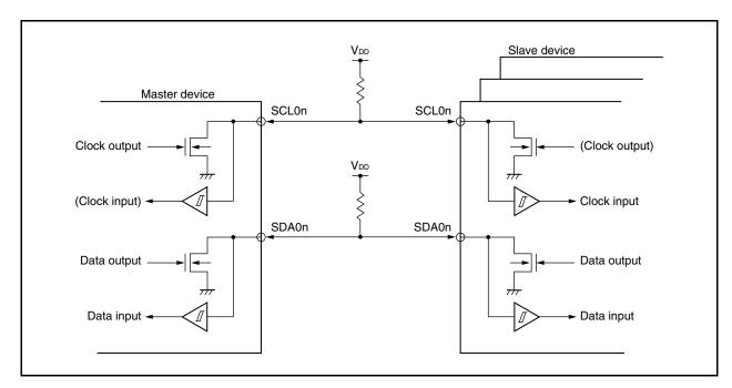
Figure 17-6. Pin Configuration Diagram
