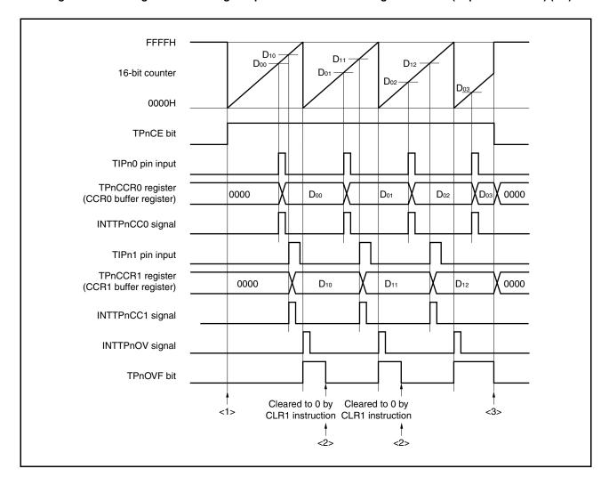
Figure 6-57. Timing and Processing of Operations in Free-Running Timer Mode (Capture Function) (2/2)
