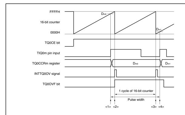
The following problem may occur when a long pulse width is measured in the free-running timer mode.
