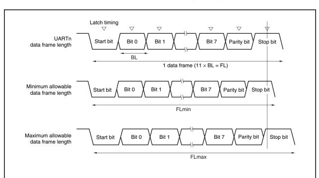
Figure 15-18. Allowable Baud Rate Range During Reception
