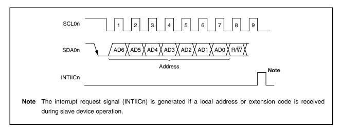
The slave address and the eighth bit, which specifies the transfer direction as described in 17.6.3 Transfer direction specification below, are written together to IIC shift register n (IICn) and then output. Received addresses are written to the IICn register.
