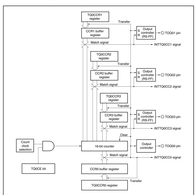
Figure 7-44. Configuration of TMQ0 in PWM Output Mode
