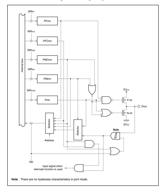
Figure 4-16. Block Diagram of Type G-16
