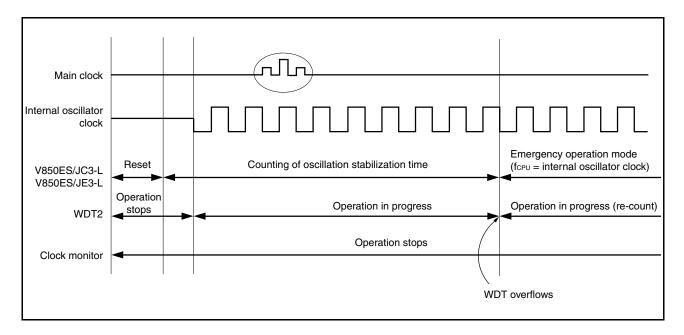
Figure 22-6. Operation Immediately After Reset Ends
