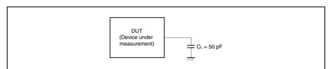
Caution If the load capacitance exceeds 50 pF due to the circuit configuration, bring the load capacitance of the device to 50 pF or less by inserting a buffer or by some other means.
