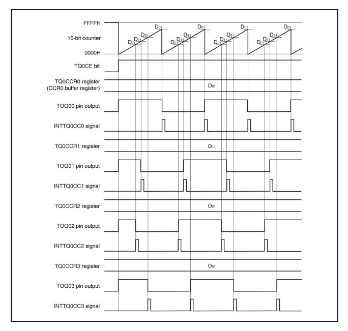
If the value of the TQ0CCRk register is greater than the value of the TQ0CCR0 register, the value of the 16-bit counter will not match the value of the TQ0CCRk register. Consequently, the INTTQ0CCk signal is not generated, nor is the output of the TQQ0k pin changed.
