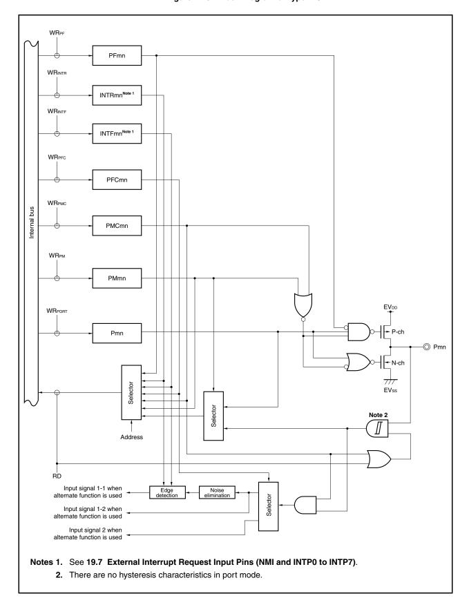
Figure 4-19. Block Diagram of Type N-3
