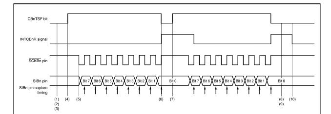
Figure 16-8. Single Transfer Mode Operation Timing (Master Mode, Reception Mode)
