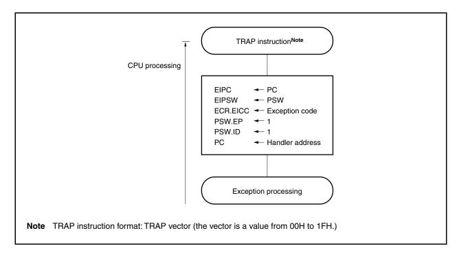
The handler address is determined by the TRAP instruction's operand (vector). If the vector is 00H to 0FH, the handler address is 00000040H, and if the vector is 10H to 1FH, the handler address is 00000050H.
