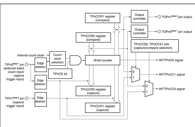
Figure 6-52. Configuration of TMPn in Free-Running Timer Mode
