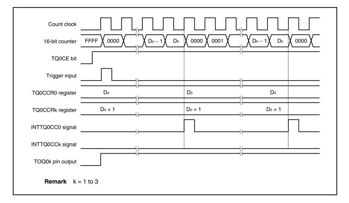
Figure 7-32. Outputting 100% PWM Waveform
