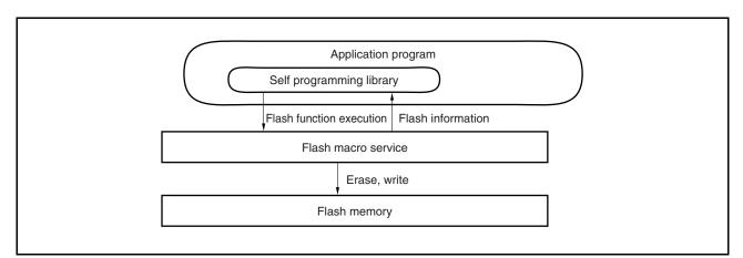
Figure 28-15. Concept of Self Programming
