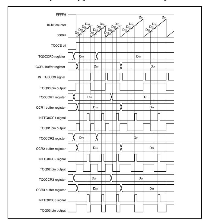
Figure 7-48. Changing PWM Waveform While Counter Is Incrementing
