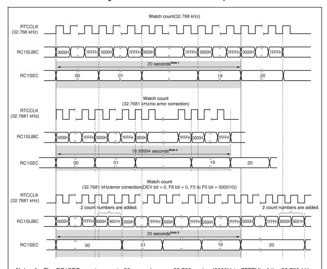
Figure 10-10. Watch Error Correction Example
