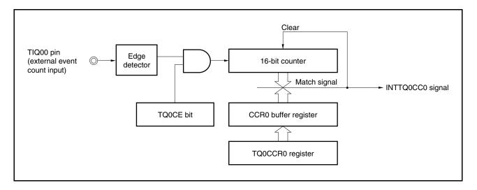
When the TQ0CE bit is set to 1, the value of the 16-bit counter is cleared from FFFFH to 0000H. The counter increments each time the valid edge of the external event count input is detected, and the value of the TQ0CCR0 register is transferred to the CCR0 buffer register.
