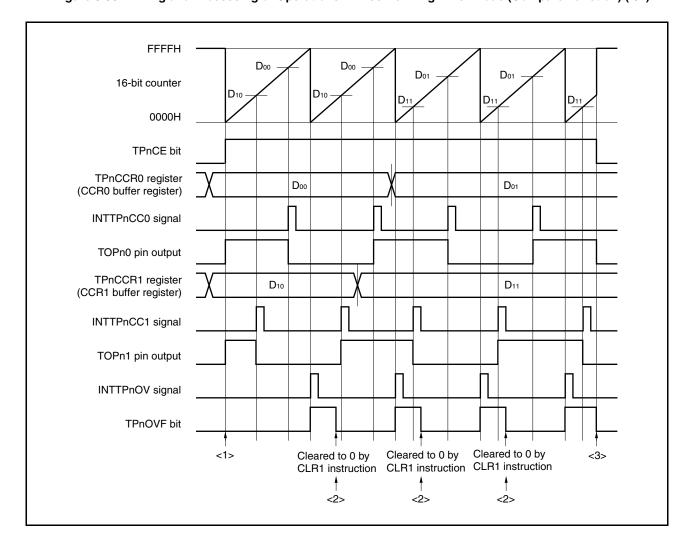
Figure 6-56. Timing and Processing of Operations in Free-Running Timer Mode (Compare Function) (2/2)
