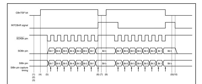
Figure 16-10. Single Transfer Mode Operation Timing (Master Mode, Transmission/Reception Mode)
