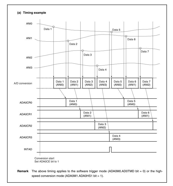
Figure 13-5. Example of Timing in Continuous Scan Mode (ADA0S Register = 03H) (1/2)
