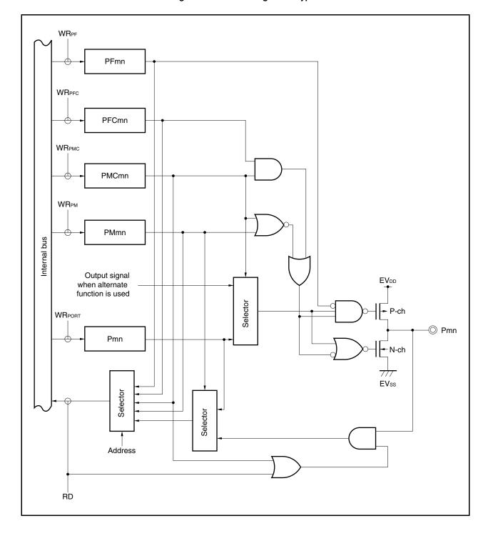
Figure 4-14. Block Diagram of Type G-14
