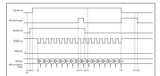
Figure 16-20. Continuous Transfer Mode Operation Timing (Master Mode, Reception Mode)
