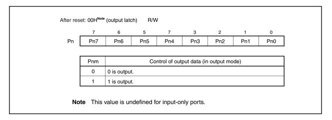
The operation when writing or reading the Pn register differs depending on the specified mode.
