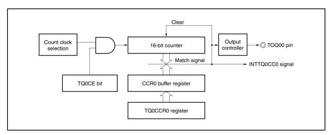
Figure 7-6. Configuration of Interval Timer
