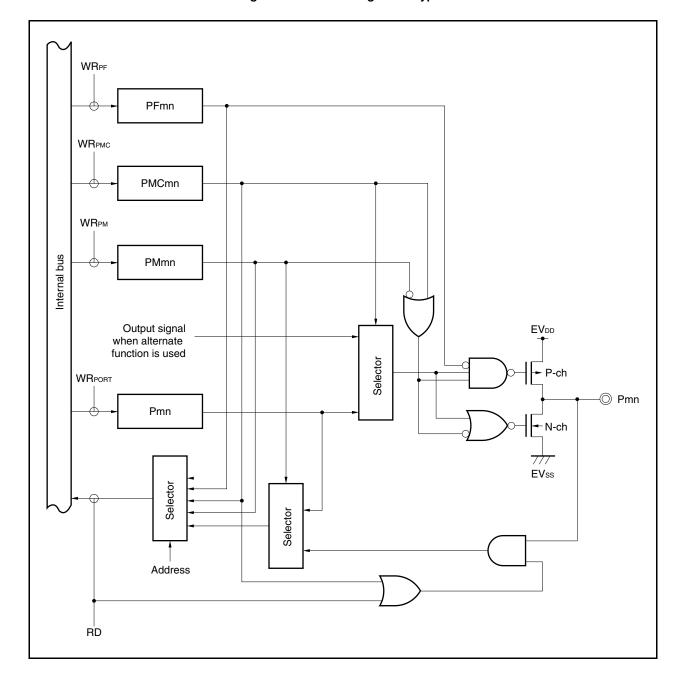
Figure 4-13. Block Diagram of Type G-13
