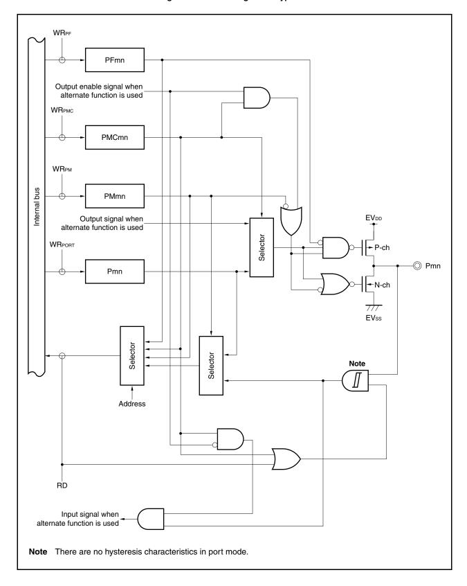
Figure 4-8. Block Diagram of Type E-3
