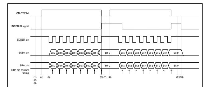
Figure 16-16. Single Transfer Mode Operation Timing (Slave Mode, Transmission/Reception Mode)
