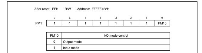
Caution When using P10 as the alternate function (ANO0 pin output), specify the input mode (PM10 bit = 1)..
