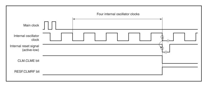
Figure 23-2. Reset Period Due to Stoppage of Main Clock Oscillation
