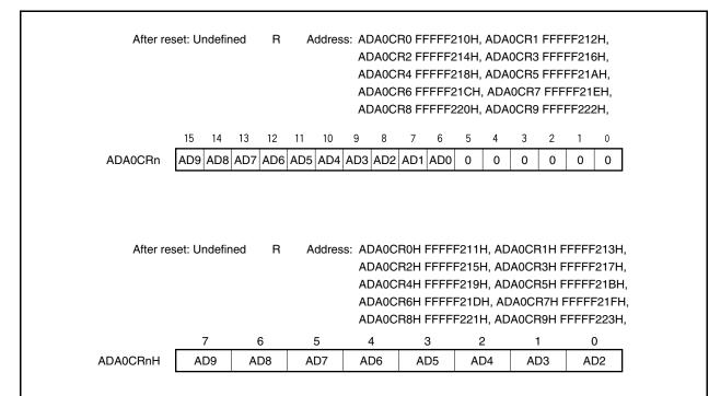
Caution A write operation to the ADA0M0 and ADA0S registers may cause the contents of the ADA0CRn register to become undefined. After conversion, read the conversion result before writing to the ADA0M0 and ADA0S registers. Correct conversion results may not be read if a sequence other than the above is used.
