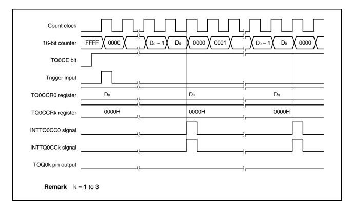
Figure 7-31. Outputting 0% PWM Waveform
