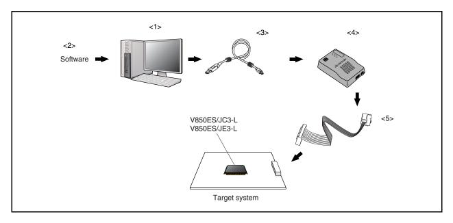
Figure A-3. On-Chip Emulation System Configuration
