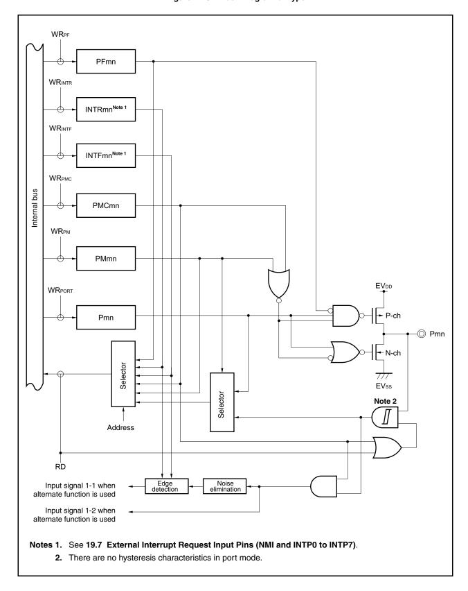
Figure 4-20. Block Diagram of Type N-4
