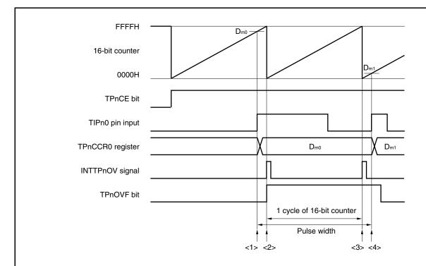
The following problem may occur when long pulse width is measured in the free-running timer mode.
