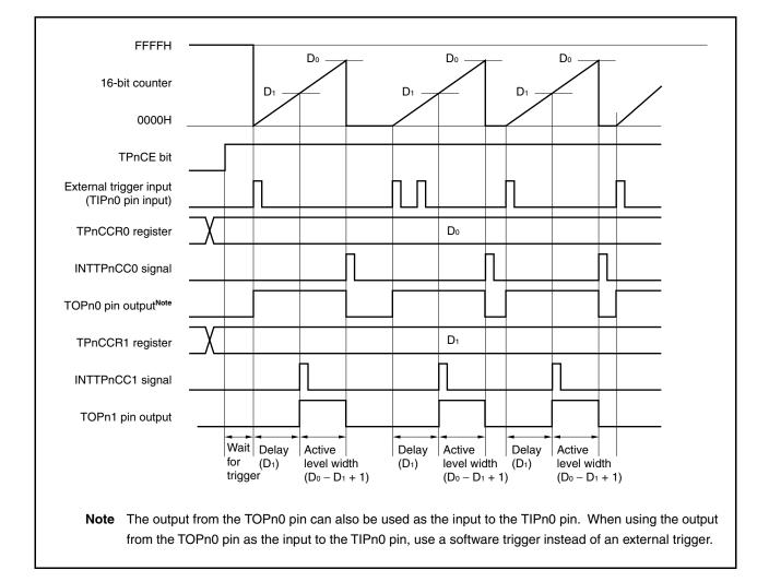
Figure 6-39. Basic Timing of Operations in One-Shot Pulse Output Mode
