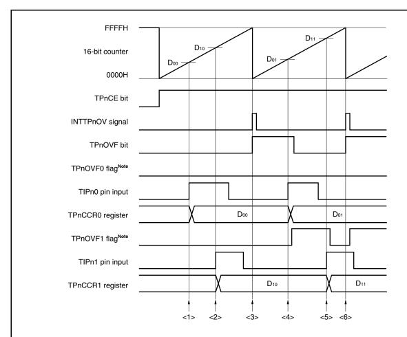
Note The TPnOVF0 and TPnOVF1 flags are set on the internal RAM by software.
