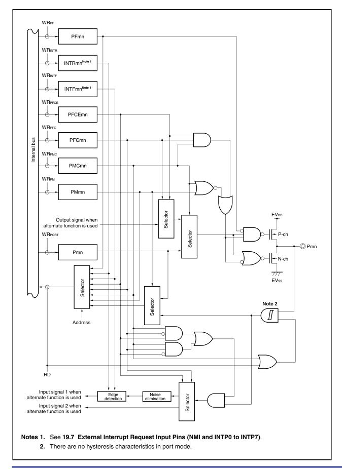
Figure 4-35. Block Diagram of Type U-24
