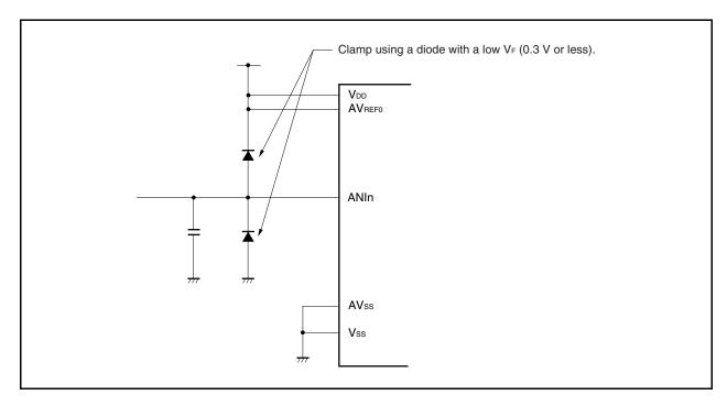
Figure 13-12. Handling of Analog Input Pin
