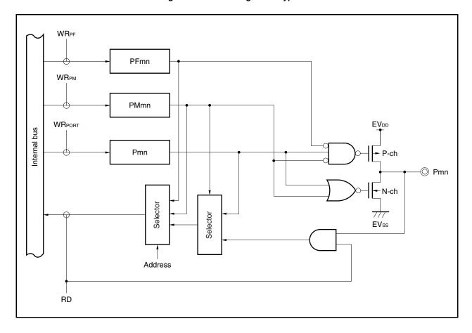
Figure 4-7. Block Diagram of Type C-1
