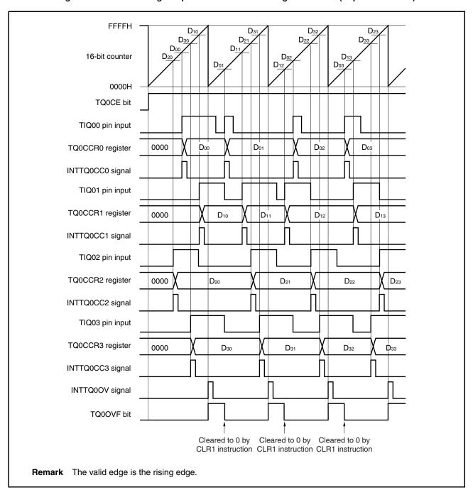
Figure 7-55. Register Settings in Free-Running Timer Mode (1/3)
