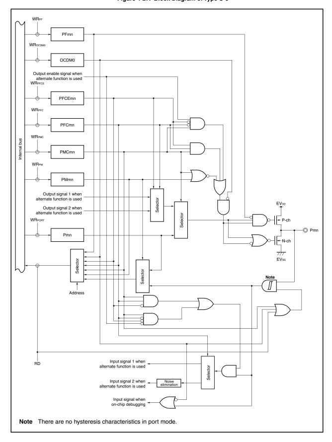
Figure 4-27. Block Diagram of Type U-9
