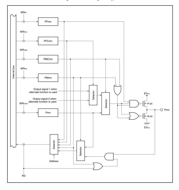
Figure 4-10. Block Diagram of Type G-3
