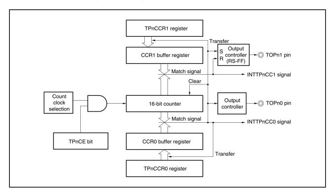
Figure 6-44. Configuration of TMPn in PWM Output Mode
