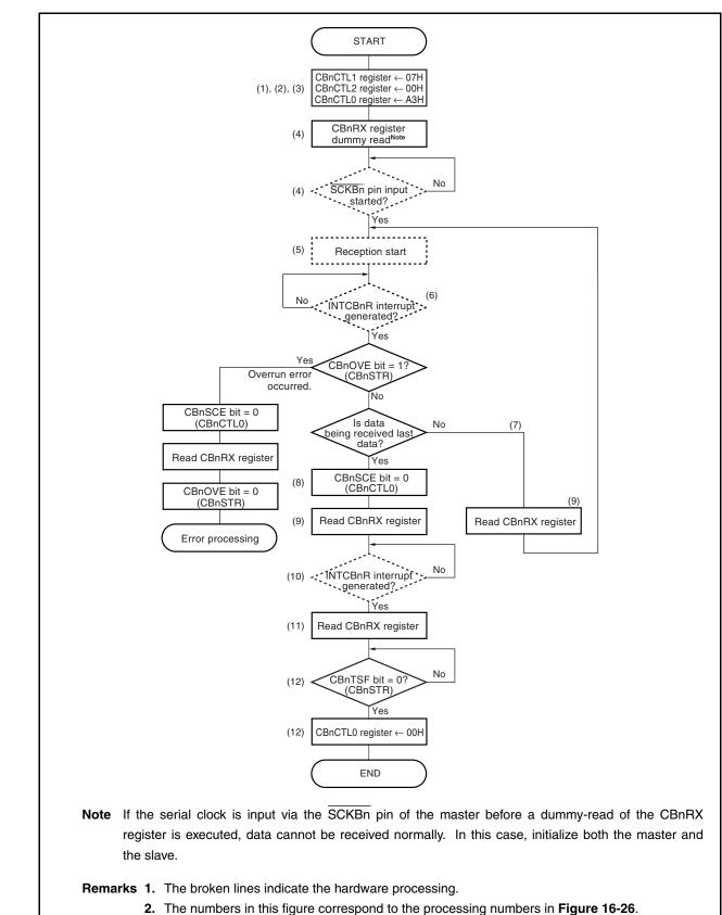
Figure 16-25. Continuous Transfer Mode Operation (Slave Mode, Reception Mode)
