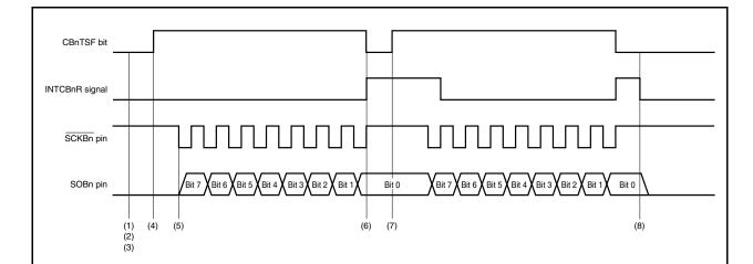
Figure 16-12. Single Transfer Mode Operation Timing (Slave Mode, Transmission Mode)
