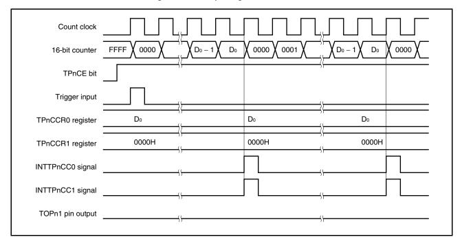
Figure 6-31. Outputting 0% PWM Waveform
