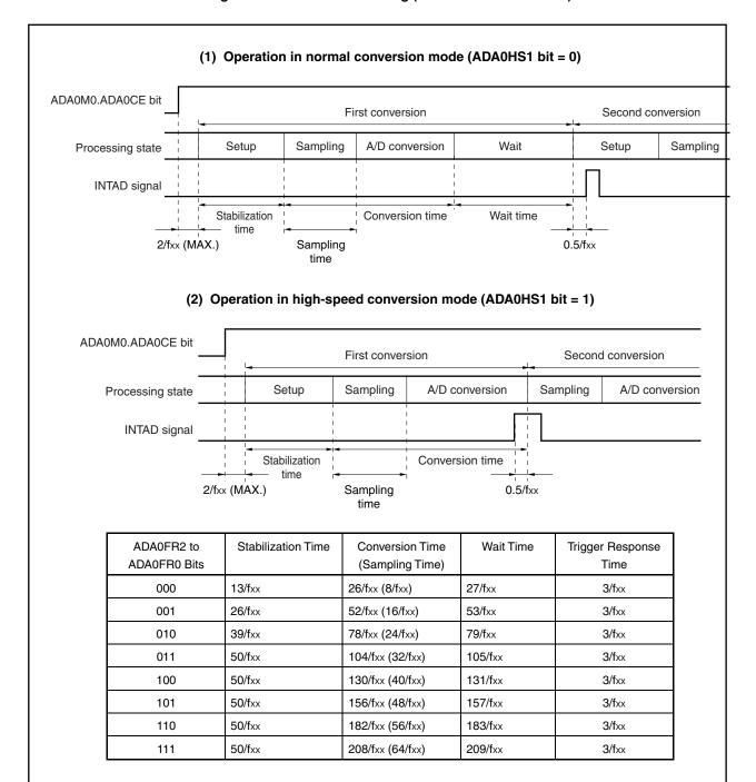
**Remark** The above timings apply to the software trigger mode. In the external trigger mode/timer trigger mode, a trigger response time is inserted.
