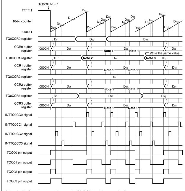
Figure 7-5. Batch Write Timing
