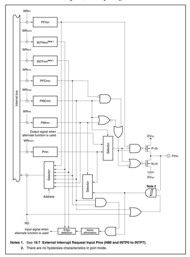
Figure 4-18. Block Diagram of Type N-2
