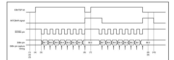
Figure 16-14. Single Transfer Mode Operation Timing (Slave Mode, Reception Mode)
