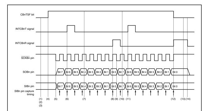
Figure 16-22. Continuous Transfer Mode Operation Timing (Master Mode, Transmission/Reception Mode) (1/2)
