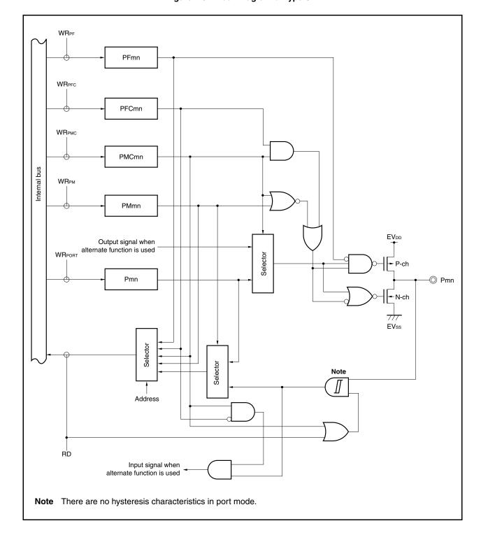
Figure 4-9. Block Diagram of Type G-1
