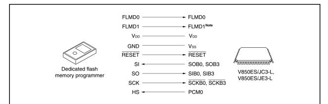
**Note** Connect the FLMD1 pin to the flash memory programmer or connect to GND via a pull-down resistor on the board.
