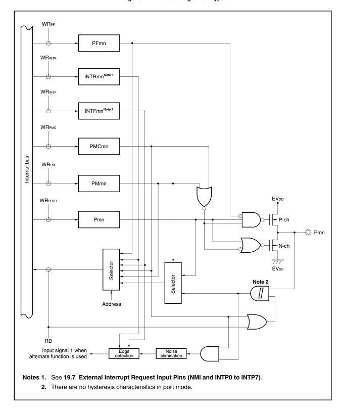
Figure 4-17. Block Diagram of Type L-1
