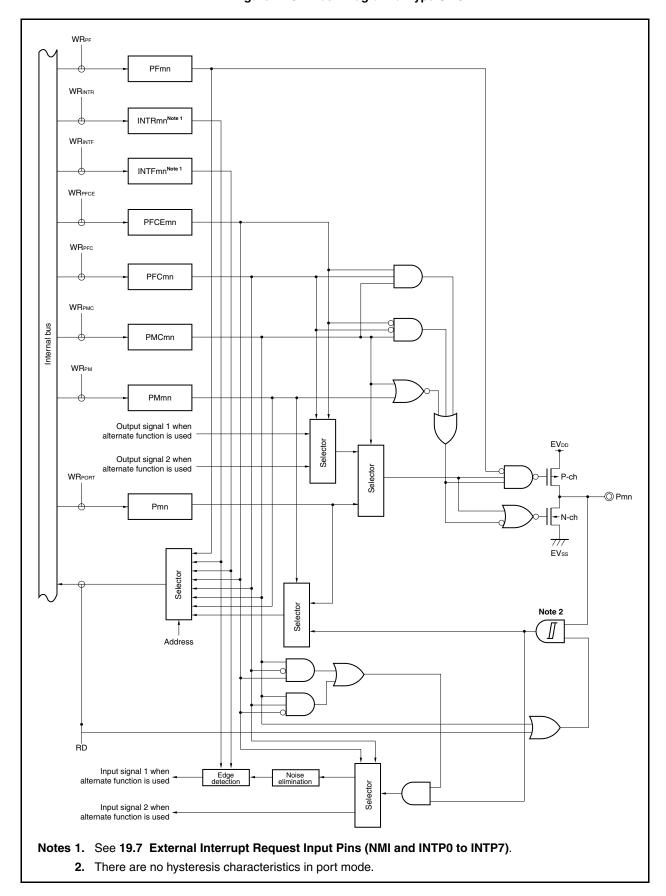
Figure 4-28. Block Diagram of Type U-15
