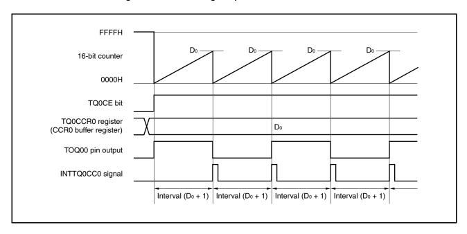
When the TQ0CE bit is set to 1, the value of the 16-bit counter is cleared from FFFFH to 0000H in synchronization with the count clock, and the counter starts incrementing. At this time, the output of the TQ000 pin is inverted and the set value of the TQ0CCR0 register is transferred to the CCR0 buffer register.
