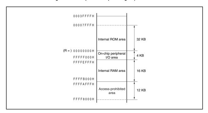
Figure 3-14. Example of Data Space Usage in  $\mu$ PD70F3840
