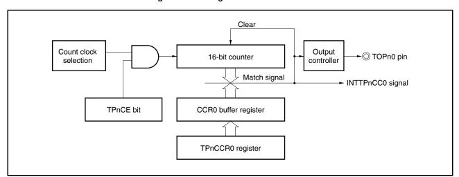
Figure 6-6. Configuration of Interval Timer
