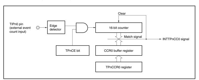
Figure 6-17. Configuration of Interval Timer in External Event Count Mode
