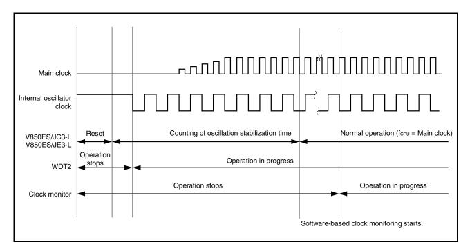
Figure 22-5. Operation Immediately After Reset Ends
