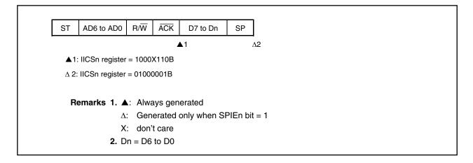
(6) When arbitration loss occurs due to low level of SDA0n pin when attempting to generate a restart condition
