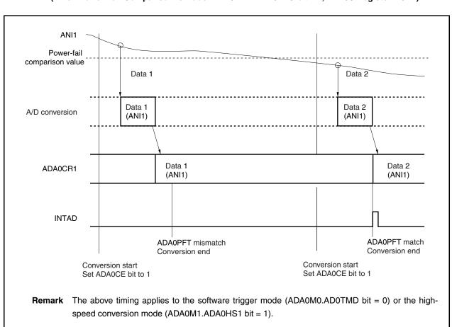
Figure 13-10. Example of Timing in One-Shot Select Mode (When Power-Fail Comparison Is Made: ADA0PFM.ADA0PFC bit = 1, ADA0S Register = 01H)
