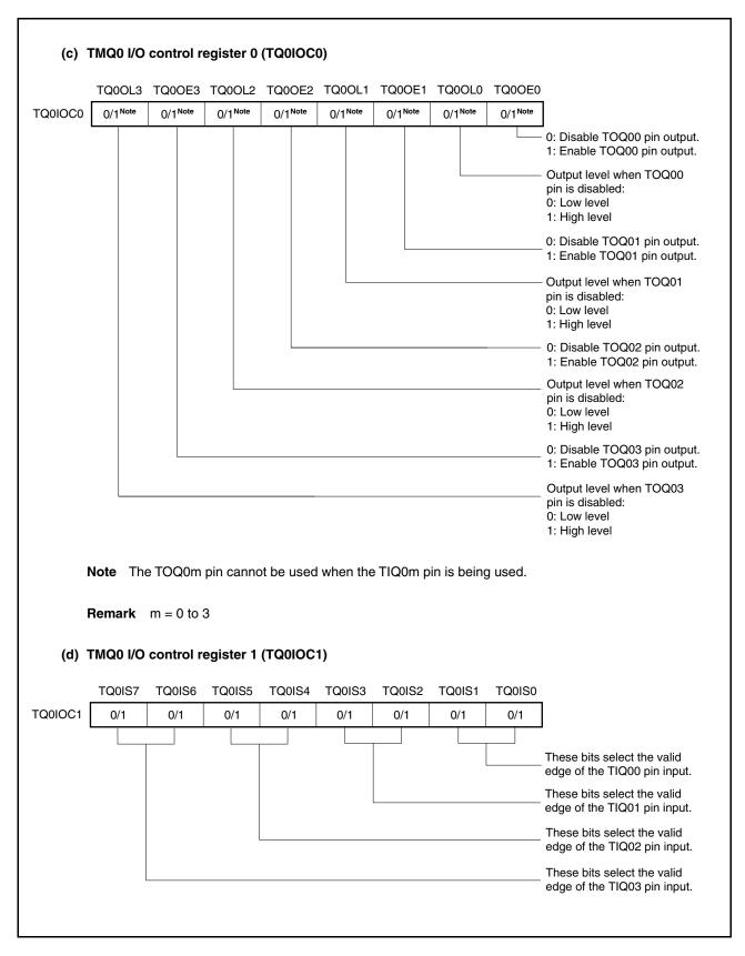
Figure 7-55. Register Settings in Free-Running Timer Mode (3/3)
