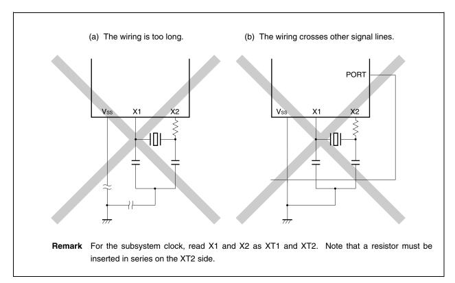
Figure 5-4. Examples of Incorrect Resonator Connections (2/2)
