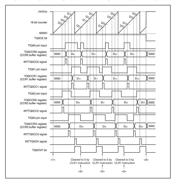
Figure 7-57. Timing and Processing of Operations in Free-Running Timer Mode (Capture Function) (2/2)
