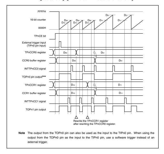
Figure 6-30. Changing PWM Waveform While Counter Is Incrementing
