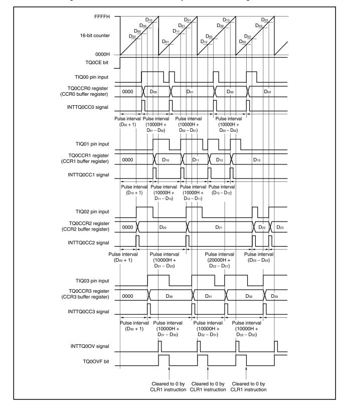
Figure 7-59. Pulse Width Measurement by TMQ0 in Free-Running Timer Mode
