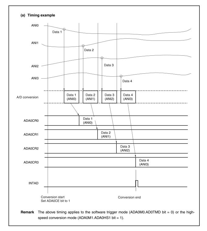
Figure 13-7. Example of Timing in One-Shot Scan Mode (ADA0S Register = 03H) (1/2)
