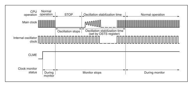
Figure 23-4. Operation in STOP Mode or After STOP Mode Is Released
