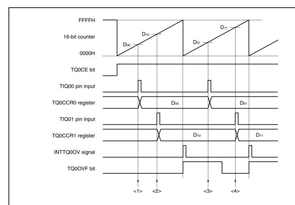
The following problem may occur when two pulse widths are measured in the free-running timer mode.
