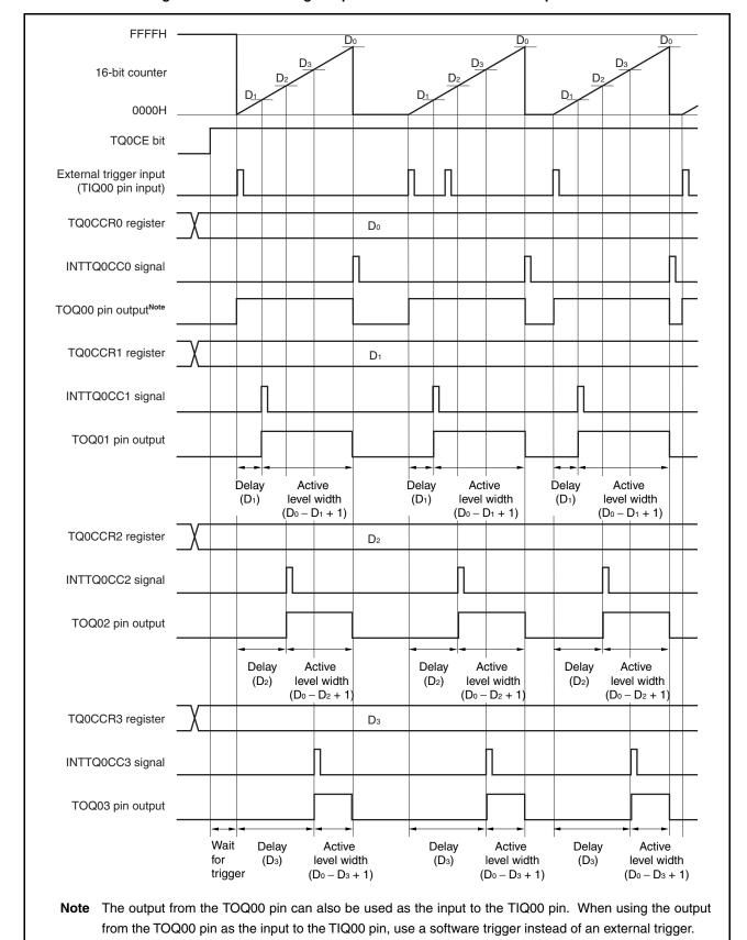
Figure 7-39. Basic Timing of Operations in One-Shot Pulse Output Mode
