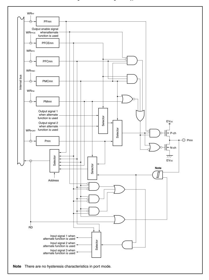
Figure 4-22. Block Diagram of Type U-1
