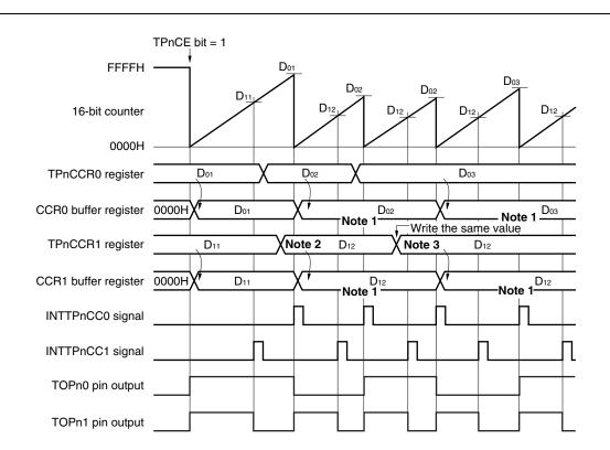
Figure 6-5. Batch Write Timing
