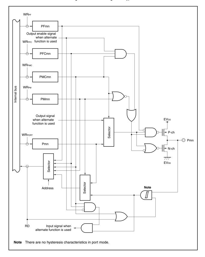
Figure 4-15. Block Diagram of Type G-15
