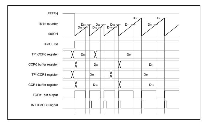
Figure 6-48. Changing PWM Waveform While Counter Is Incrementing
