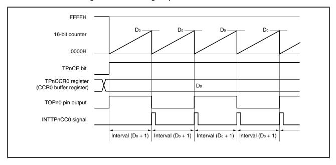
When the TPnCE bit is set to 1, the value of the 16-bit counter is cleared from FFFFH to 0000H in synchronization with the count clock, and the counter starts incrementing. At this time, the output of the TOPn0 pin is inverted and the set value of the TPnCCR0 register is transferred to the CCR0 buffer register.
