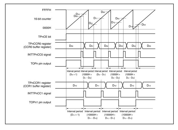
Figure 6-58. Interval Operation of TMPn in Free-Running Timer Mode
