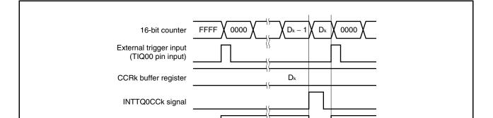
Figure 7-33. Detection of Trigger Immediately After INTTQ0CCk Signal Was Generated
