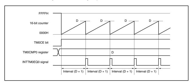
An example of the register settings when the interval timer mode is used is shown in the figure below.
