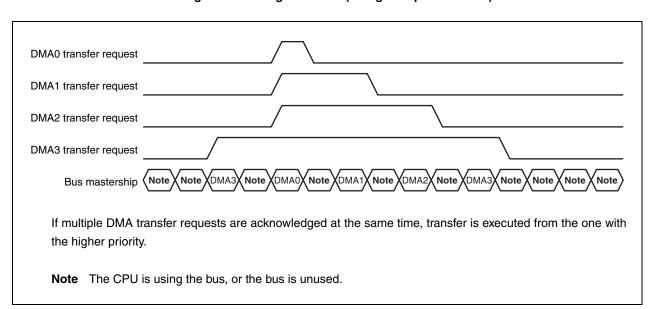
Figure 18-3. Single Transfer (Using Multiple Channels)
