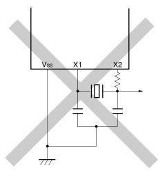
**Remark** For the subsystem clock, read X1 and X2 as XT1 and XT2. Note that a resistor must be inserted in series on the XT2 side.
