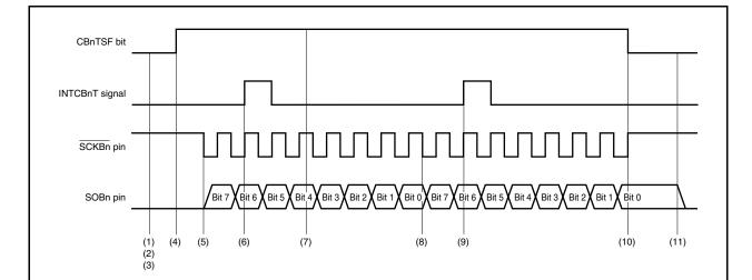
Figure 16-24. Continuous Transfer Mode Operation Timing (Slave Mode, Transmission Mode)
