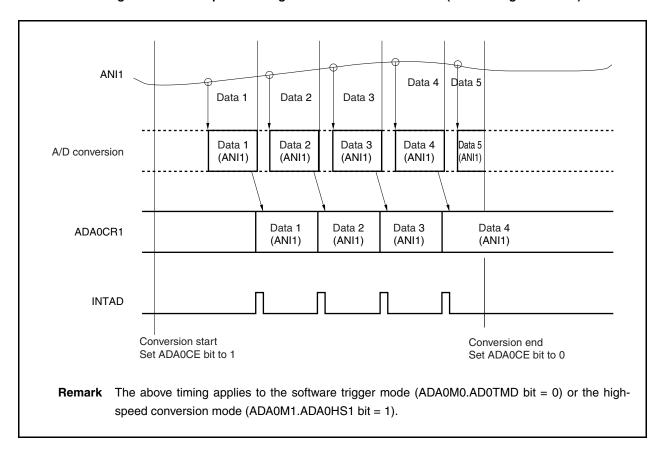
Figure 13-4. Example of Timing in Continuous Select Mode (ADA0S Register = 01H)
