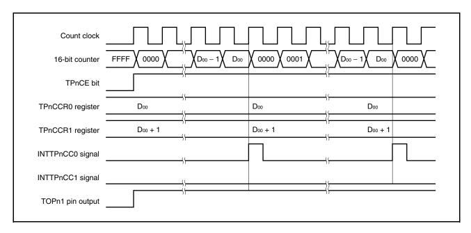
Figure 6-50. Outputting 100% PWM Waveform
