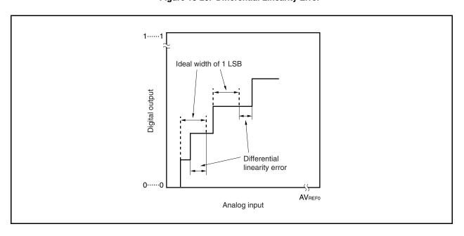
Figure 13-20. Differential Linearity Error
