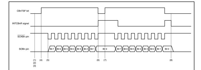
Figure 16-6. Single Transfer Mode Operation Timing (Master Mode, Transmission Mode)
