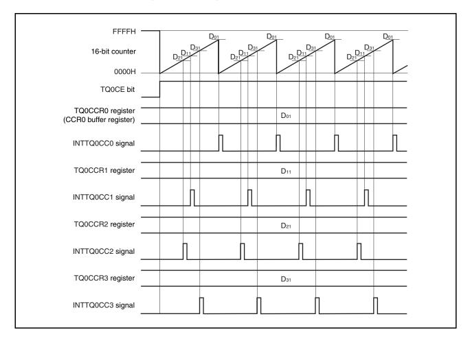
If the value of the TQ0CCRk register is greater than the value of the TQ0CCR0 register, the value of the 16-bit counter will not match the value of the TQ0CCRk register and the INTTQ0CCk signal will not be generated. A chart showing the timing of operations when the value of the TQ0CCRk register ( $D_{k1}$ ) is greater than the value of the TQ0CCR0 register ( $D_{01}$ ) is shown below.
