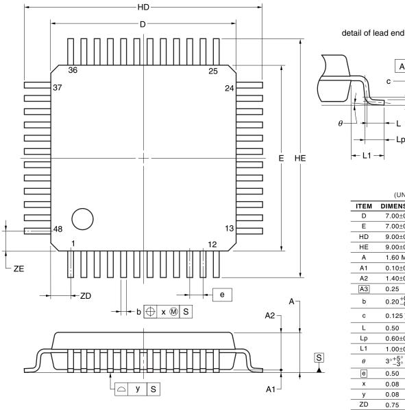
NOTE Each lead centerline is located within 0.08 mm of its true position at maximum material condition.
