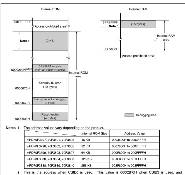
Figure 29-5. Memory Spaces Where Debug Monitor Programs Are Allocated
