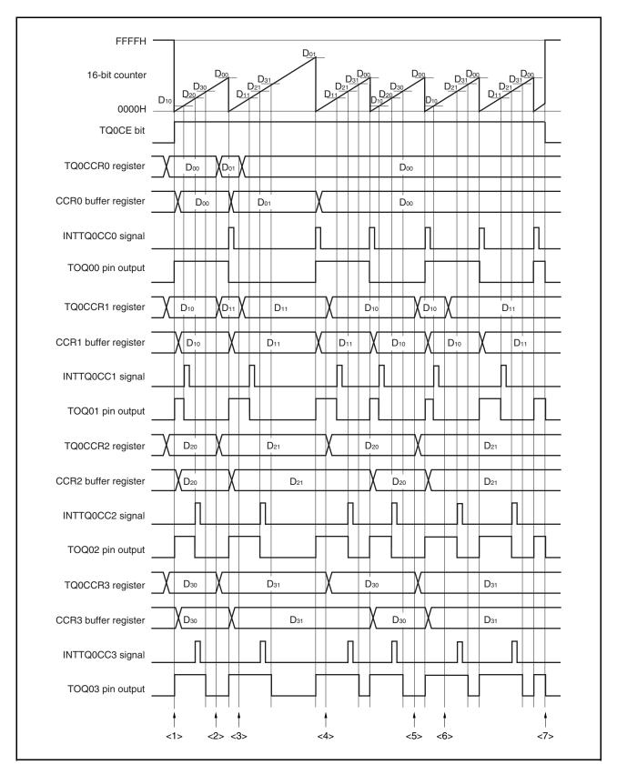
Figure 7-47. Timing and Processing of Operations in PWM Output Mode (2/2)
