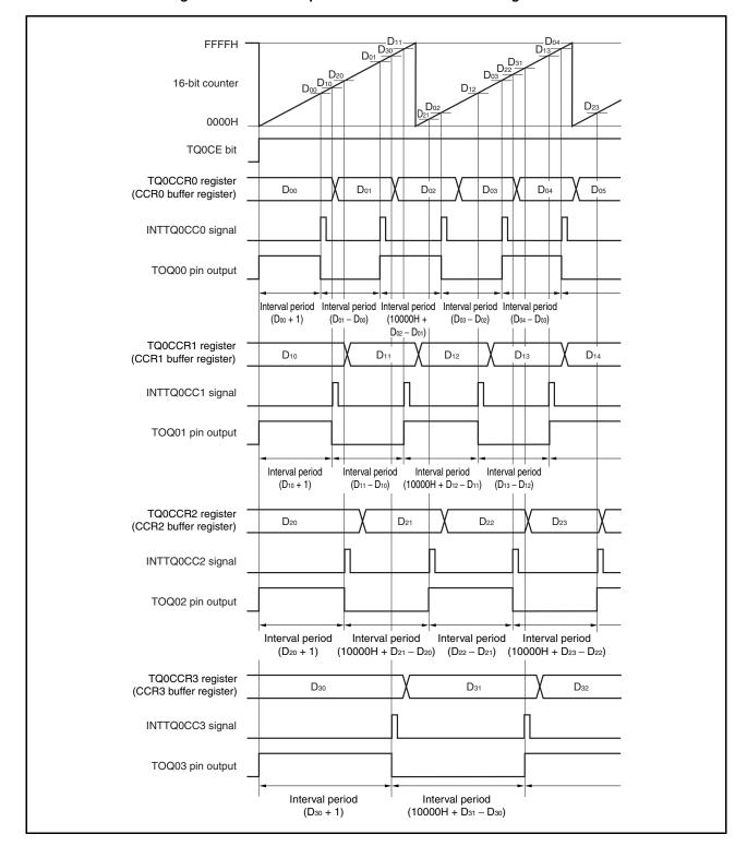
Figure 7-58. Interval Operation of TMQ0 in Free-Running Timer Mode
