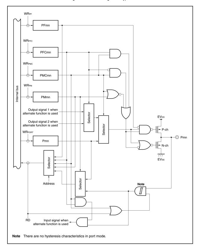
Figure 4-12. Block Diagram of Type G-12
