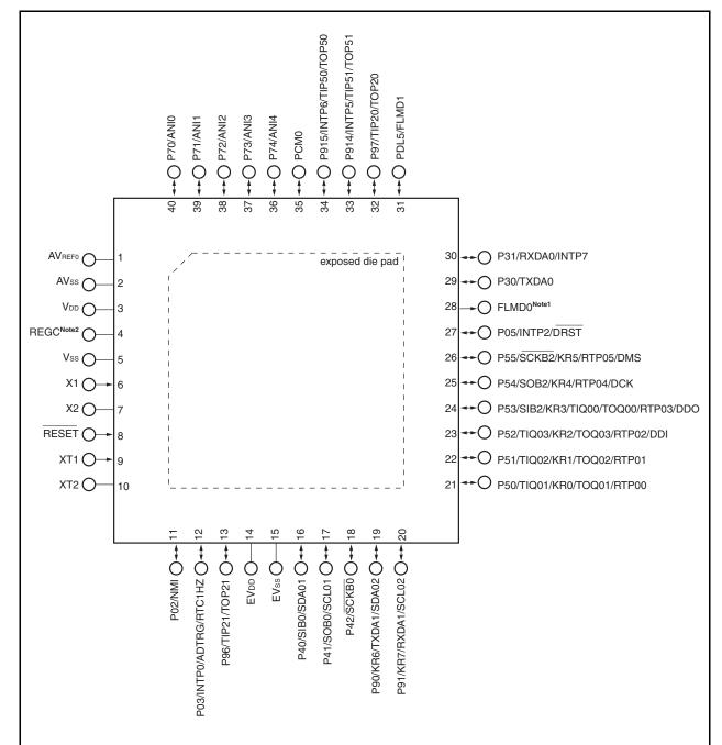
Notes 1. The FLMD0 pin is used in flash programming. Connect this pin to Vss in the normal operation mode.
