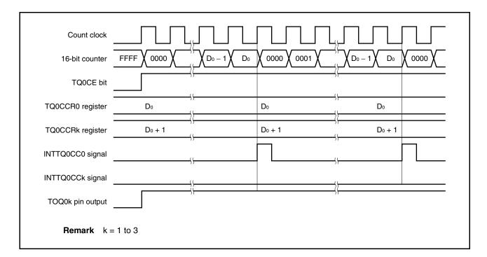
Figure 7-50. Outputting 100% PWM Waveform
