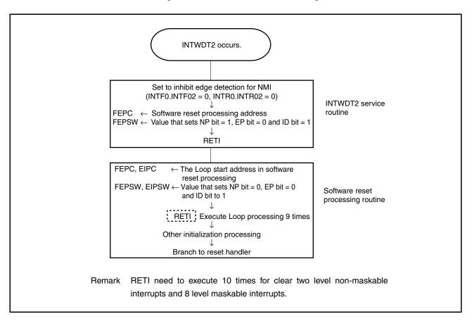
Figure 19-4. Software Reset Processing
