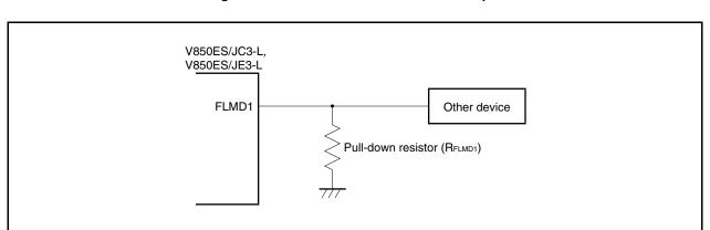
Figure 28-10. FLMD1 Pin Connection Example
