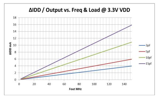
Figure 1. Total Current = Disabled Current +  $\triangle$ IDD Fout1 +  $\triangle$ IDD Fout2
