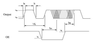
Figure 3. OE Function and Output Waveform
