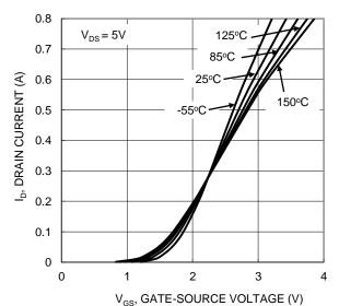
Figure 2. Typical Transfer Characteristic
