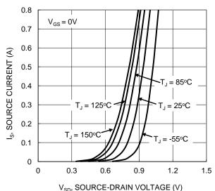
Figure 9. Diode Forward Voltage vs. Current
