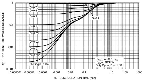
Figure 13. Transient Thermal Resistance
