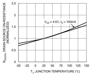
Figure 6. On-Resistance Variation with Junction Temperature
