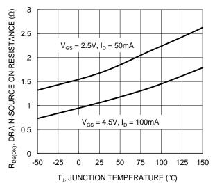
Figue 7. On-Resistance Variation with Junction Temperature
