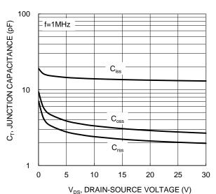
Figure 10. Typical Junction Capacitance
