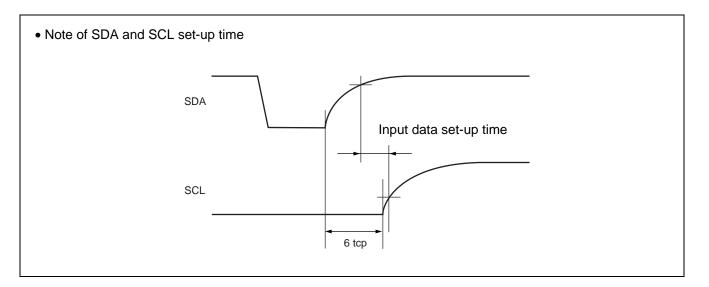
Note : The rating of the input data set-up time in the device connected to the bus cannot be satisfied depending on the load capacitance or pull-up resistor. Be sure to adjust the pull-up resistor of SDA and SCL if the rating of the input data set-up time cannot be satisfied.
