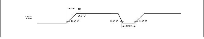
Note : Sudden change of power supply voltage may activate the power-on reset function. When changing power supply voltages during operation, raise the power smoothly by suppressing variation of voltages as shown below.
