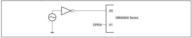
Please set XOA = GND and X1A = open without subclock mode. The following figure shows the using sample.
