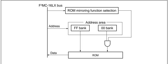
Note : Do not access to ROM mirroring function selection register in the middle of the operation of the address 008000<sub>H</sub> to 00FFFF<sub>H</sub>.
