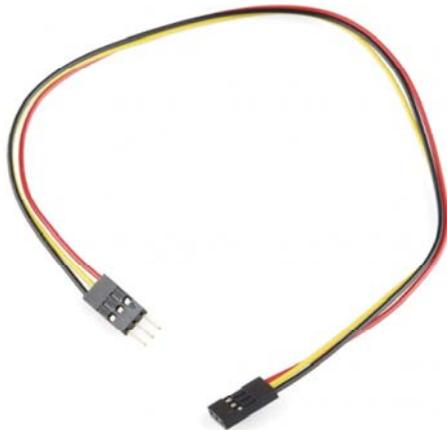
The Feedback Cable is made of three separate wires – colored red, yellow, and black. Red should always be connected to the + pin, black to the – pin, yellow will pass the signal through.
