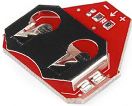
The Power Block runs on a single **20mm coin cell battery**, which optimally provides around 3V, and should last for quite a while. The LogicBlocks can work at voltages between 2 and 5V, and they consume very little current.
