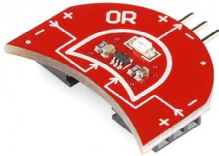
You can connect either an **Input Block** or the output from another **Gate Block** to either of the two inputs. This male output connector can be plugged into either the input of another gate, or a **Power Block**.
