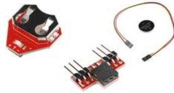
There's also a **Splitter** LogicBlock, which simply divides one input into two outputs. It doesn't perform any operation on the signal, just passes it through. This'll come in handy when you create more complicated digital logic circuits which require one input to run into two or more logic gates.
