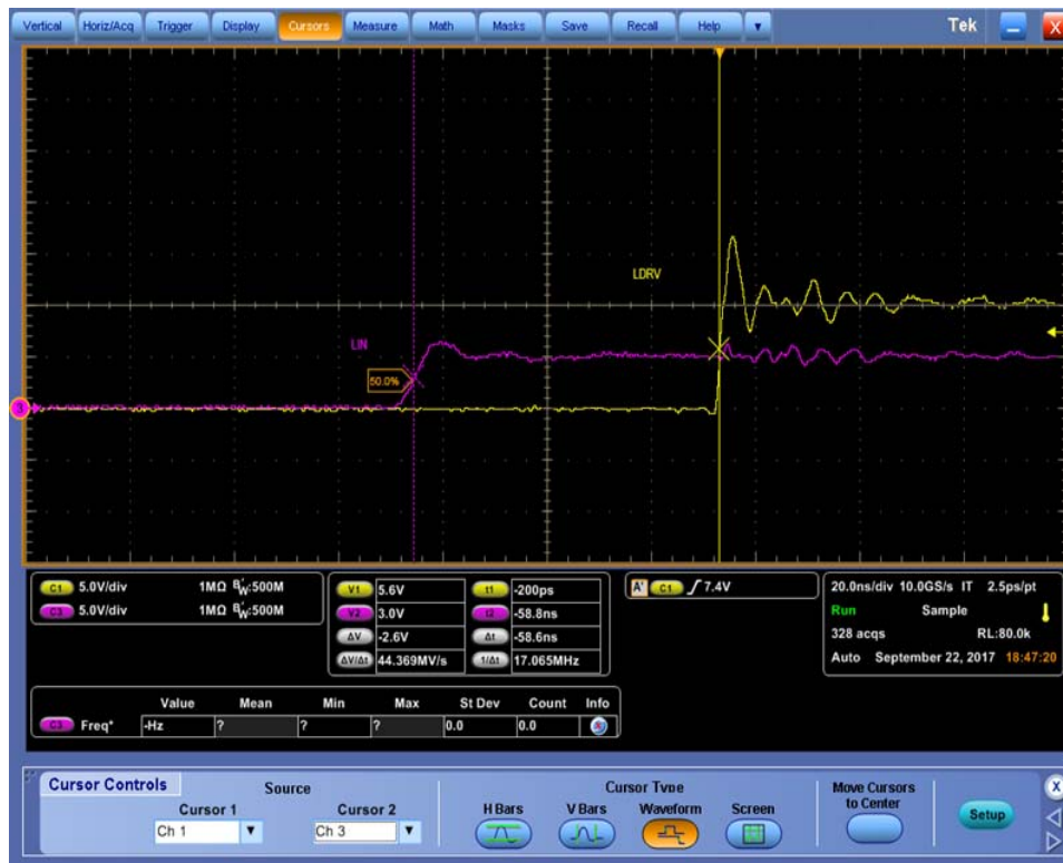
Figure 30. Low Side Turn-ON Propagation Delay (NCP51530A)
