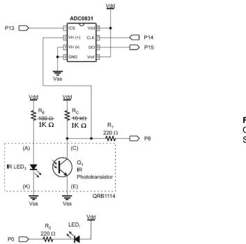
Figure 0-1 Opto-Reflective Switch Monitoring
