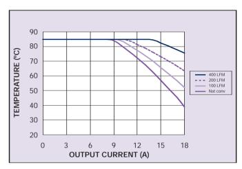
Figure 1 - Safe Operating Area Vin = 5 V, Output Voltage = 3.3 V (See Note A)
